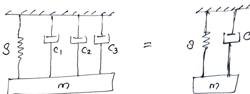
The effective damping coefficient of the dampers in parallel is the sum of their individual damping coefficients.
