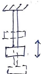
When the particles of the shaft (or disc) moves parallel to the axis of the shaft, is known as longitudinal vibrations.
