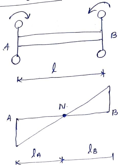
$$f_{nA} = \frac{1}{2\pi} \sqrt{\frac{CJ}{l_A I_A}}, \quad f_{nB} = \frac{1}{2\pi} \sqrt{\frac{CJ}{l_B I_B}}$$
