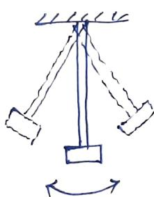
When the particles of the shaft (or disc) moves approximately perpendicular to the axis of the shaft, is known as transverse vibrations.
