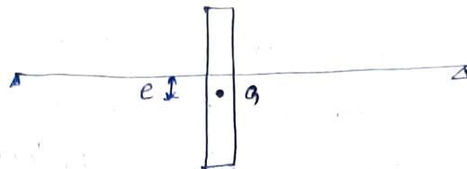
\* The speed at which the shaft runs so that the additional deflection of the shaft from the axis of rotation becomes infinite, is known as critical (or) whirling speed.
