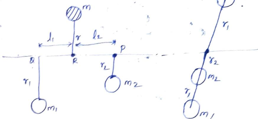
Here Net dynamic force  $\overset{\text{on Net force}}{\cancel{F_c}}$  acting on the shaft is equal to zero. [ ]
