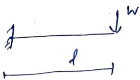
$$= \frac{100 \times 9.81 \times 300^3}{3 \times 200 \times 10^9 \times \frac{\pi^2}{64} \times 50^4} = 0.0147 \text{ mm}$$
