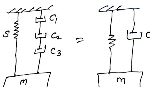
The reciprocal of the effective damping coefficient of the dampers in series is the sum of the reciprocal of their individual damping coefficients.
