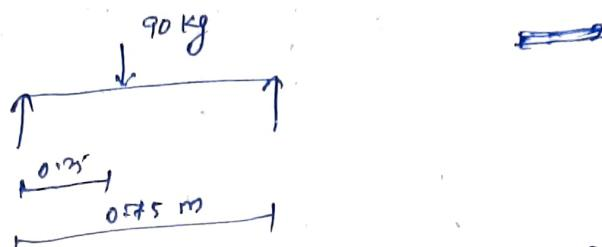
$$\delta = \frac{\omega a b^2}{3EI l} = \frac{90 \times 9.81 \times 0.25^2 \times 0.5^2}{3 \times 200 \times 10^9 \times \frac{\pi}{64} \times 0.05^4 \times 0.75}$$
