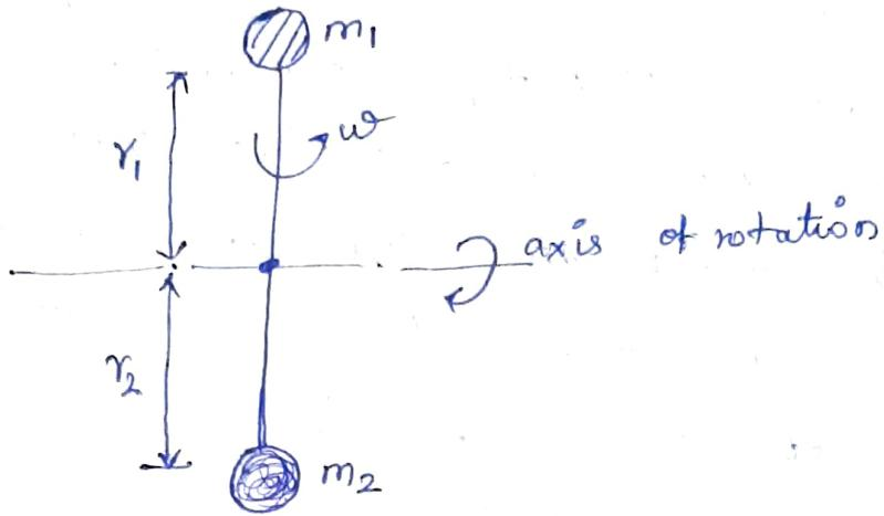
centrifugal force due to first mass,  $F_{C_1} = m_1 \omega^2 r_1$
