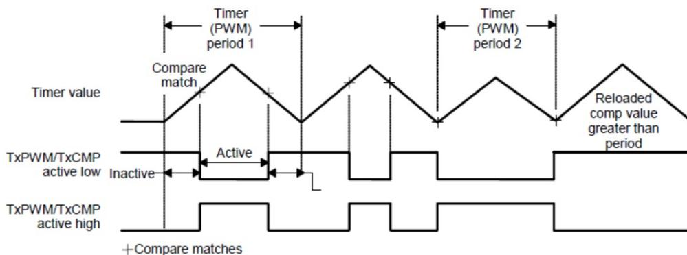
Figure 3 Symmetric timer waveform from continuous up/down count mode.
