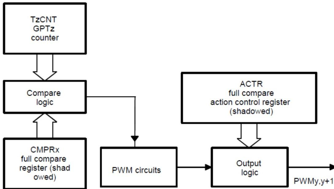
Figure 4 Compare unit block diagram.
