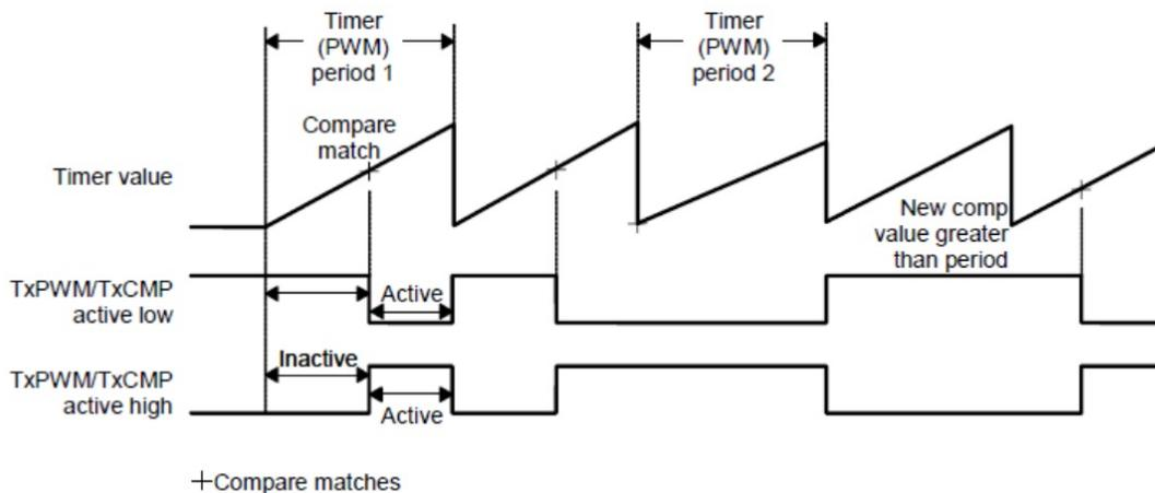
Figure 2 Asymmetric timer waveform generated by a GP timer in continuous up-count mode.
