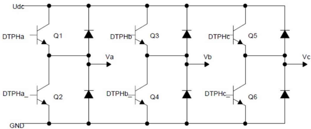
Figure 5 Basic three-phase inverter circuit.
