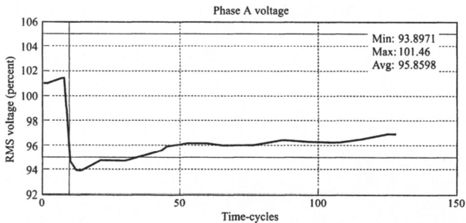
**Fig 5. Voltage sag due to induction motor starting.**
