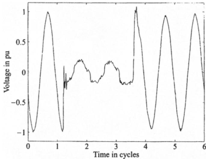
**Fig 4. Voltage sag due to short circuit fault.**
