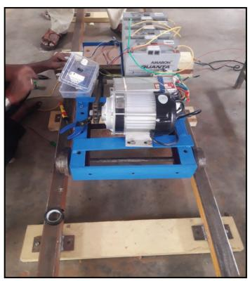
Microcontroller then sends the signal to the motor and the motor drives the wheels. A separate switch has been given for moving the vehicle to move in the opposite direction. The entire setup has been developed and successfully tested to move in both linear and circular motion.
