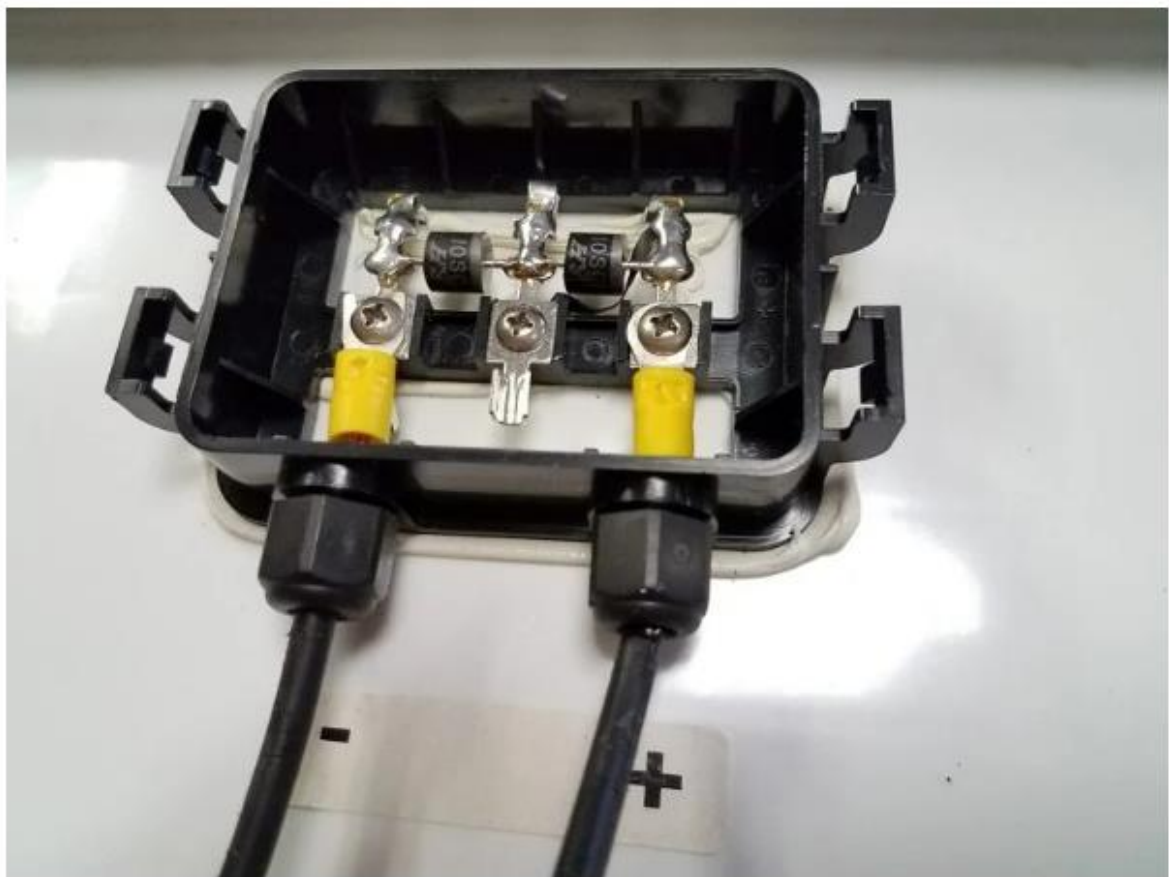
Diode stripe (cathode) pointing to positive
